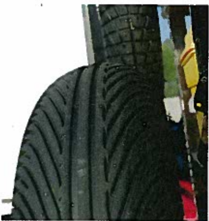
Dunlop's standard front rain tire (top) works in conjunction with the rear to evacuate water as quickly as possible and actually provide knee-dragging lean angles under full wet conditions. In drying conditions, the soft tread blocks flex and disintegrate from the heat buildup, making for an ill-handling bike.
